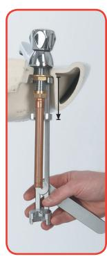
Sliding jaws dropped to allow tightening of tap back nuts without having to turn off the water supply or drain the system
