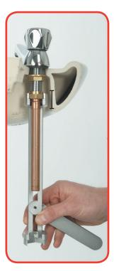
Sliding jaws locked in position to allow tightening / removal of pipe nut.
